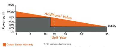
2 Out linear warranty with 2.5% degradation in the 1st year and less than 0.55% degradation each year from 2nd year to 30th year
